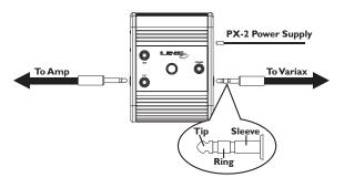
Powering your Variax Acoustic with the XPS is easy. Use the included TRS cable (meaning "Tip-Ring-Sleeve" or also simply known as a "stereo" cable) to connect the Variax Acoustic to the INPUT jack of the XPS. Connect the PX-2 power supply to the XPS POWER jack, and use a standard mono guitar cable to connect the XPS's 1/4-inch OUTPUT to your acoustic amp or mixer.
