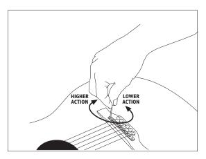
Variax Acoustic leaves the factory adjusted for playability across a wide range of playing styles. The bridge saddle height can be adjusted to optimize playability for a particular style. If you are familiar with this kind of adjustment, use the supplied Allen wrench to raise or lower the bridge saddle screws as shown. As with neck adjustment, if you are unfamiliar with this kind of adjustment, ask your local guitar shop to refer you to a qualified guitar tech.
