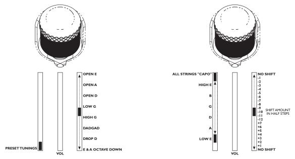
We made it easy to get to some of the most commonly used alternate tunings. First, enter the Alternate Tuning Set-Up mode with a quick double press on the model select knob. The LED will flash red-green-red-green to let you know you are in this mode. With the bottom (COMPRESSOR) slider all the way down, choose the tuning you want with the top (MIC) slider.
